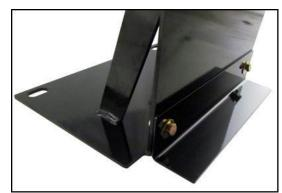
3. Install (A) Magnum Buddy Seat floor bracket on 2 factory seat bolts. Secure with (E) flat washer and locking nuts
