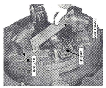
Use special gauge to adjust transmission clutch lever height on early models
