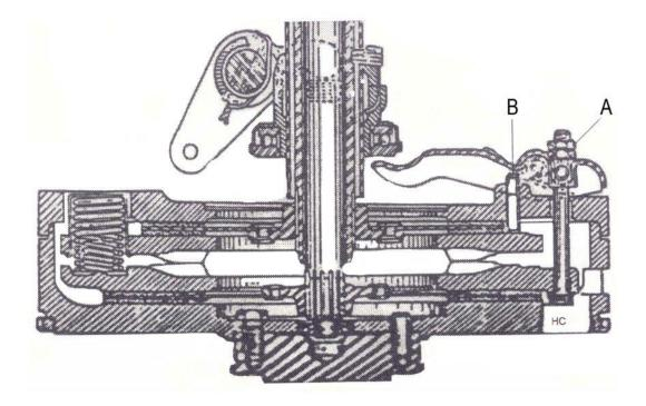
After clutch assembly have been bolted to flywheel a release lever adjustment must be done. Loosen adjusting nuts (A) evenly until release levers contact PTO clutch push pins (B). Tighten adjusting nuts 2-1/2 turns and then secure by tightening jam nuts
