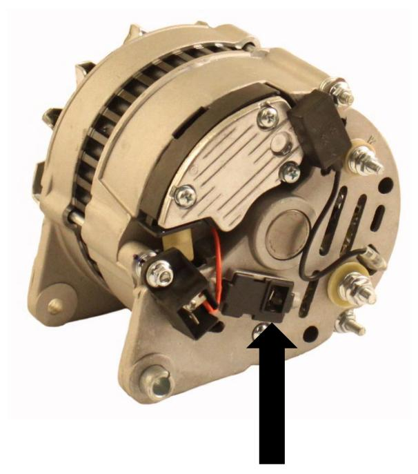
For three spade connection, remove this plastic cover
