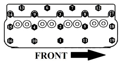
After Run-in re-torque head gasket by loosening each nut/bolt in sequence ½ turn and re-torqueing to above spec.
