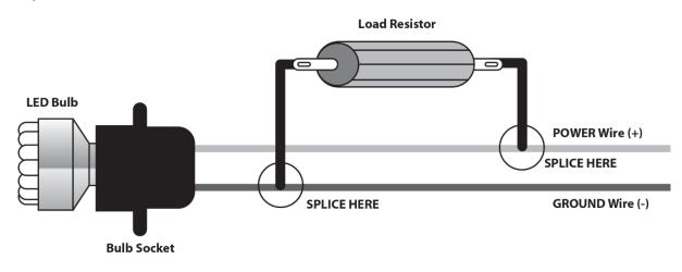
When there are more than two wires coming out of the turn signal bulb, you will need to isolate the turn signal wires for the resistor to work properly. Determine which two wires are for the turn signal by using a voltage meter or by referring to the manual.
